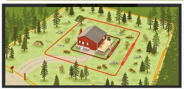
Defensible space is the area around a home or other structure that has been modified to reduce fire hazards. In this area, natural and manmade fuels are treated, cleared or reduced to slow the spread of wildfire.
